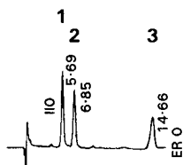
FIG. 1. Typical HPLC elution pattern of a standard mixture of adenine nucleotides (2 \mu M). 1. ATP (retention time 5.7 min); 2. ADP (6.9 min); 3. AMP (14.7 min).
